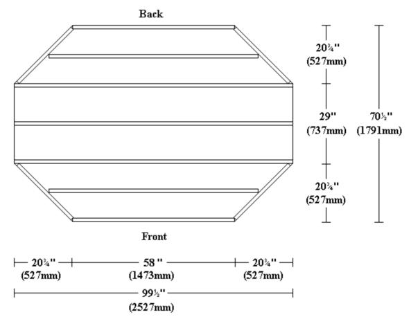
NB:- Floor joists run side to side.
